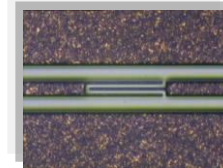
High frequency capacitor 80 GHz
