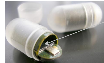
Electronic pill showing the IPD (8 mm diameter x 17 mm long)
